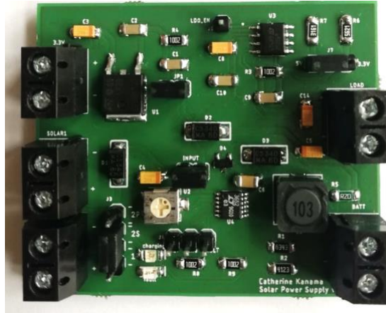
Figure 29: Soldered solar power supply board
