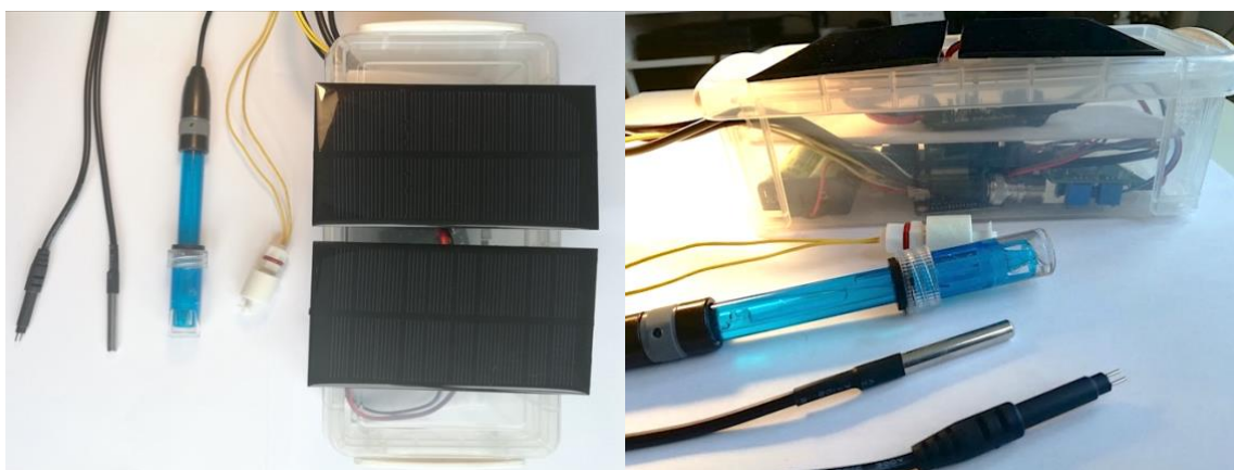
Figure 33: Top and side view of the solar powered water monitoring device
